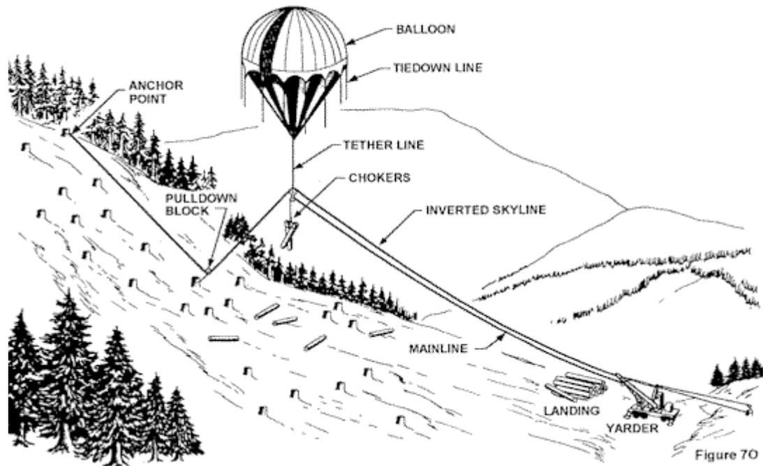
Figure 7. Balloon Extraction – Haulback Configuration. Picture from [9].
