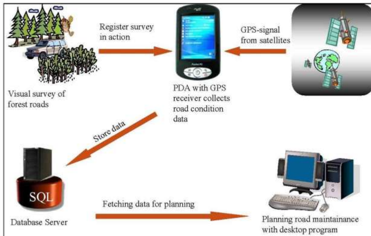
Figure 4-3 Principle for road survey with pocket PC.
