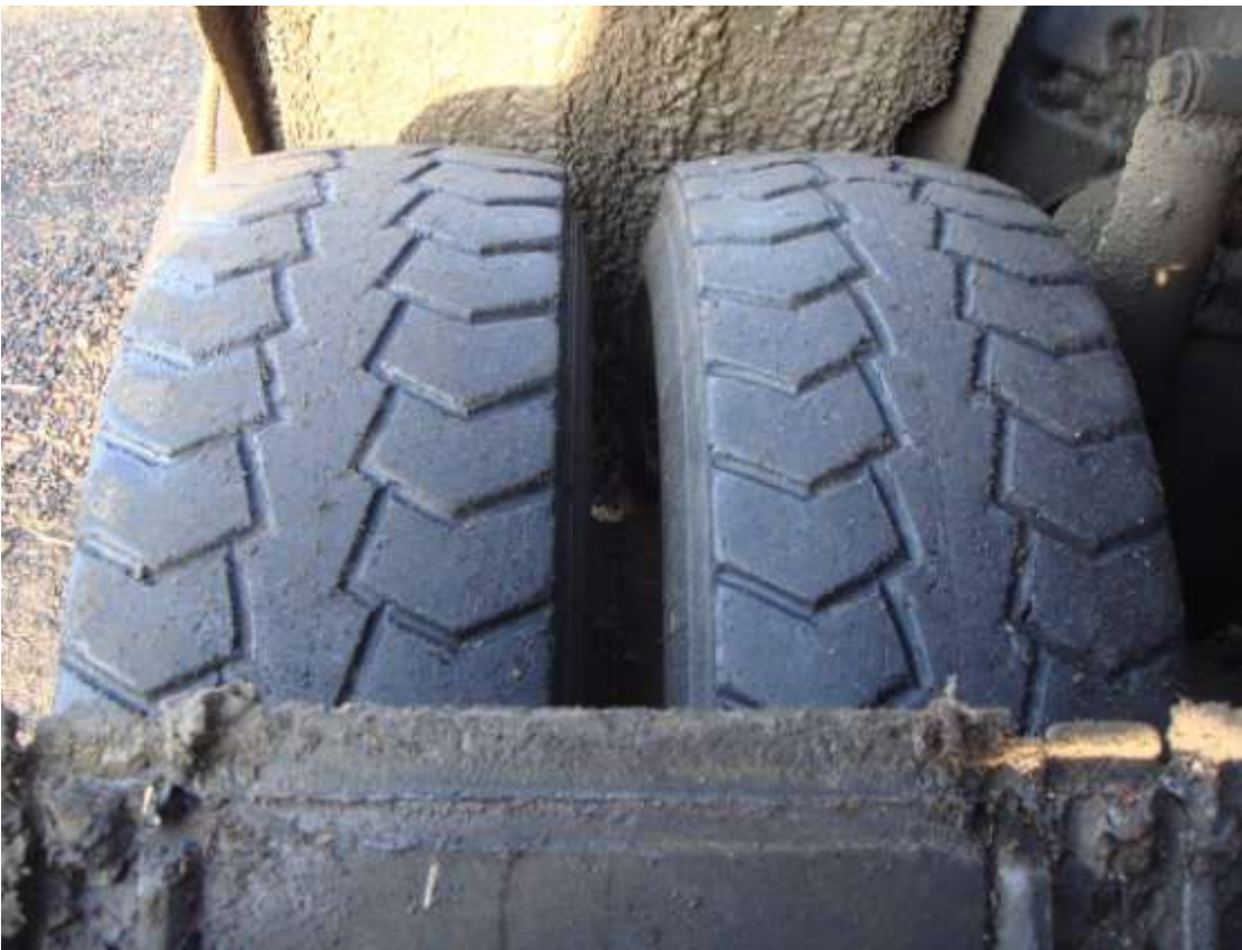
Photographs of drive tyres at 108,000km (Tyres regrooved at 79,000km)
