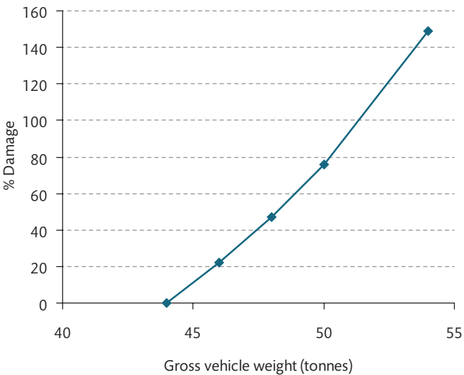
Figure 12 Percentage road damage against gross vehicle weight (from Road haulage of round timber – the Timber Transport Forum).
