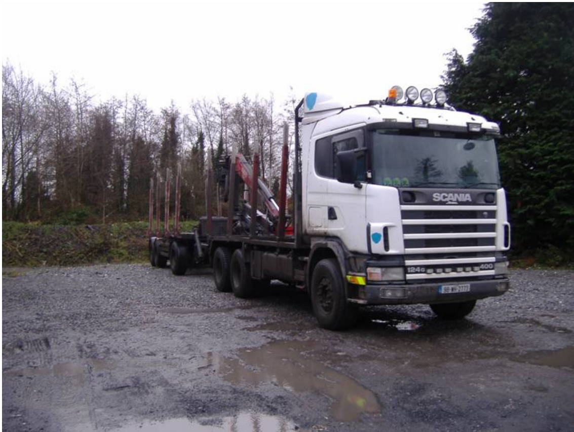
Fig. (4). Scania 124 (400) rigid + trailer + crane configuration.
