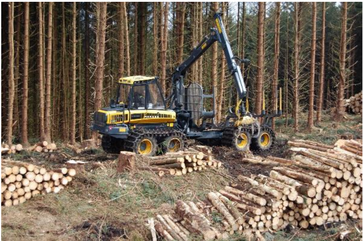
Figure 8 A forwarder collects cut logs and takes them to a stack on a forest road. Photo Confor
