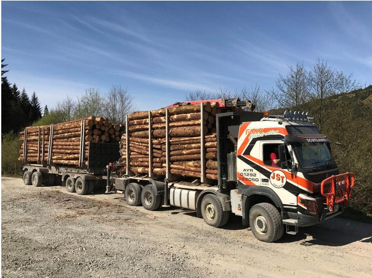
Figure 15 This 8 axle in-forest haulage vehicle can carry a 50t payload of timber Photo JST Services Ltd
