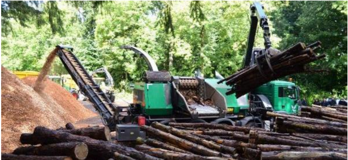
Figure 9 Mobile chipper processing logs for biomass fuel, Photo Confor
