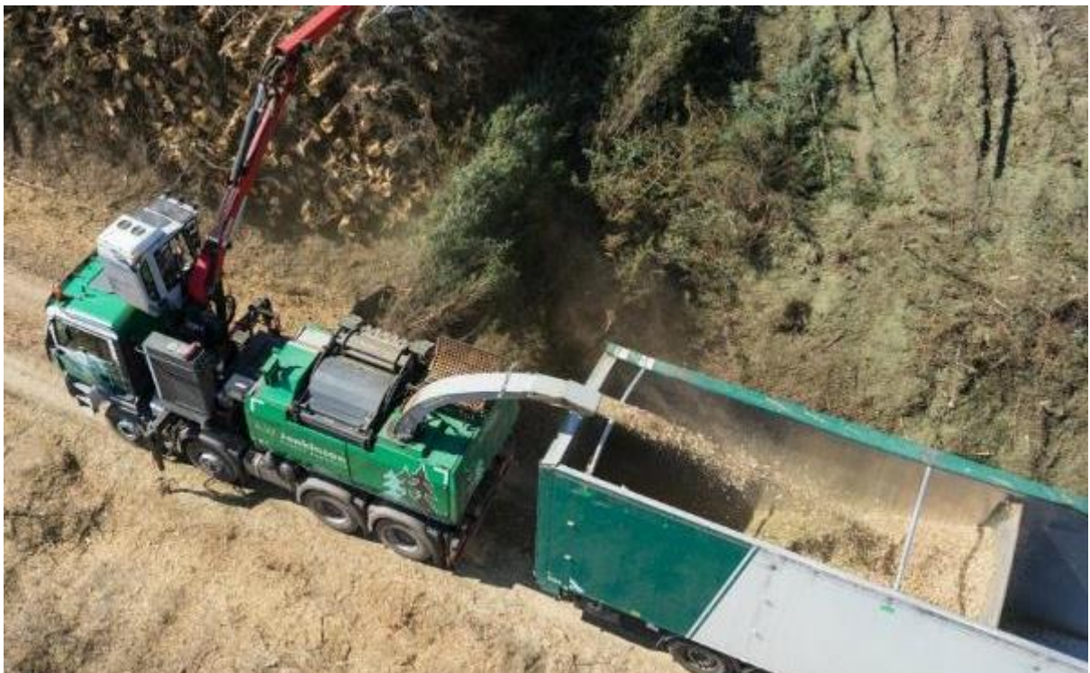
Figure 10 This chipper uses 3000 litres of red diesel a week to chip 800-1000 tonnes of timber Photo Mulholland Media
