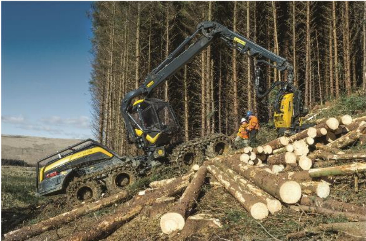
Figure 7 A timber harvester can process (fell, de-limb and cross cut) 200 tonnes of timber per day and typically costs £400,000 Photo Confor
