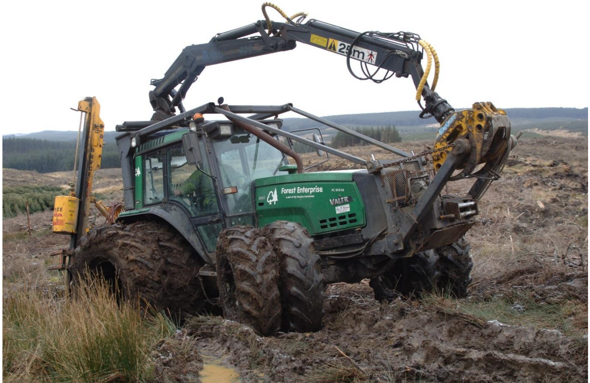
Figure 6 A tractor being used for installing deer fencing Photos Forestry Commission Crown Copyright
