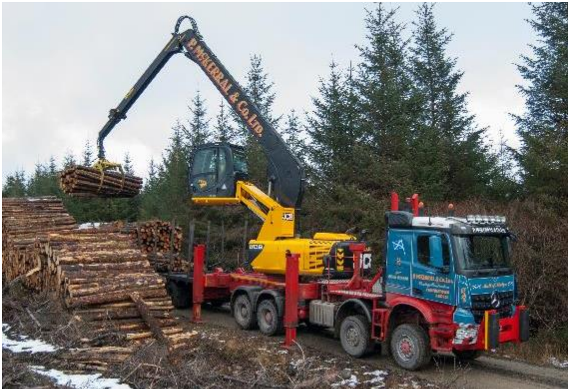
Figure 18 This independent mobile crane runs on red diesel and is used to load road-going lorries with timber, Photo Peter McKerral
