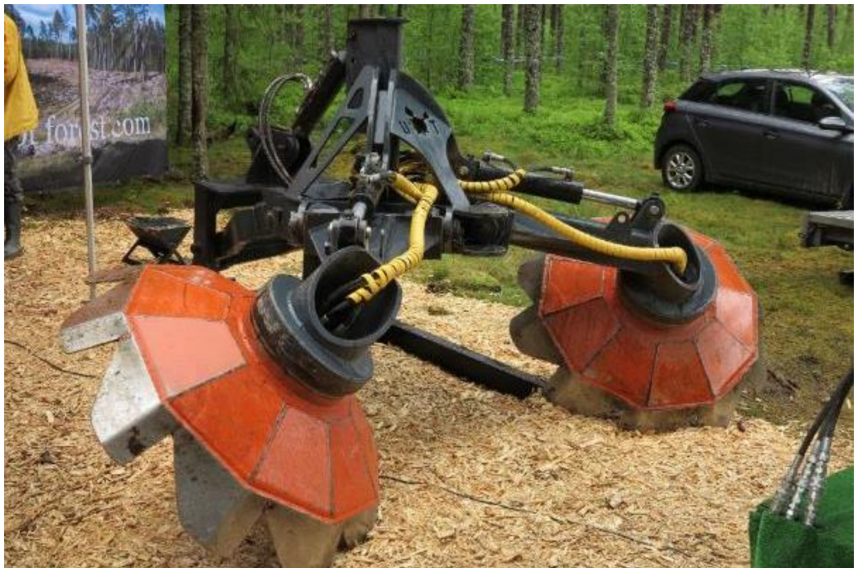
Figure 5 A scarifier is towed behind a tractor and scrapes planting sites
