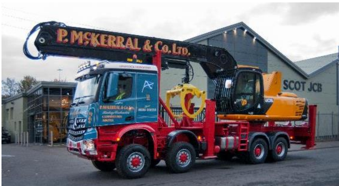
Figure 17 This independent mobile crane runs on red diesel and is used to load road-going lorries with timber, Photo Peter McKerral
