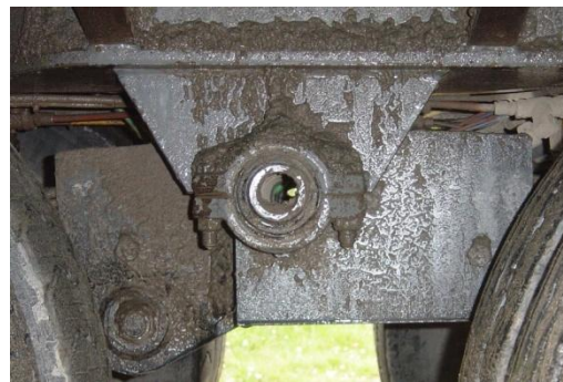
Illustration 12: Photos showing balance beam arrangement on trailer compared to bogie
