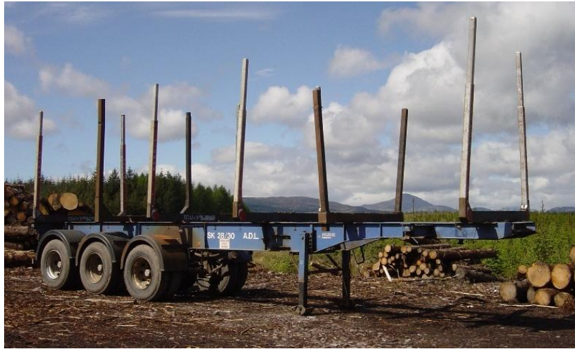
Illustration 16: Skeletal trailer parked at a transshipment point
