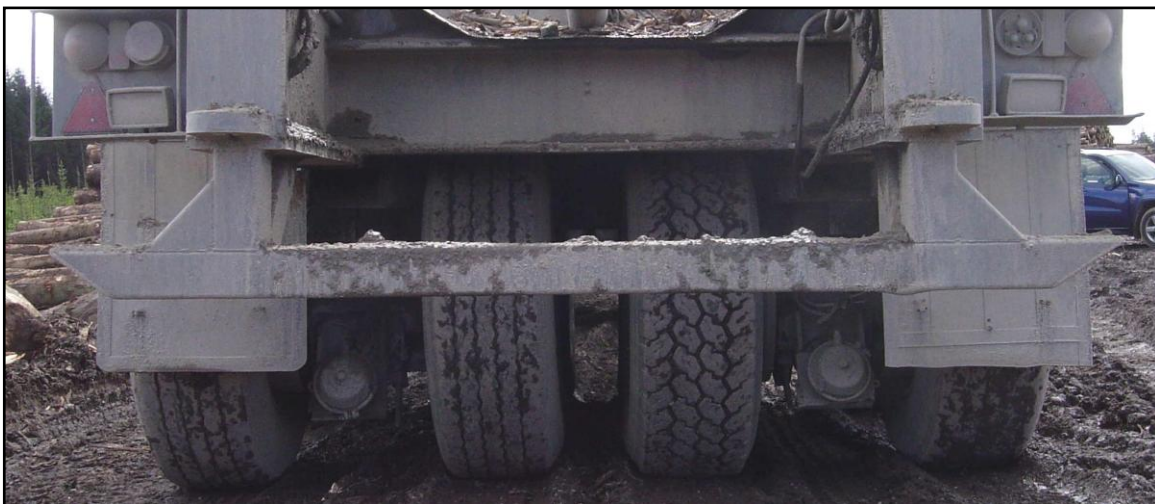
Illustration 5: A rear view of the King trailer. Note the articulation and position of the wheels
