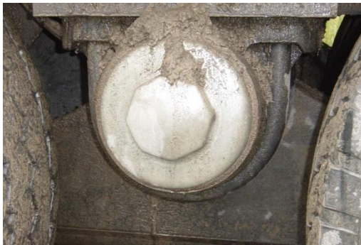
Illustration 12: Photos showing balance beam arrangement on trailer compared to bogie
