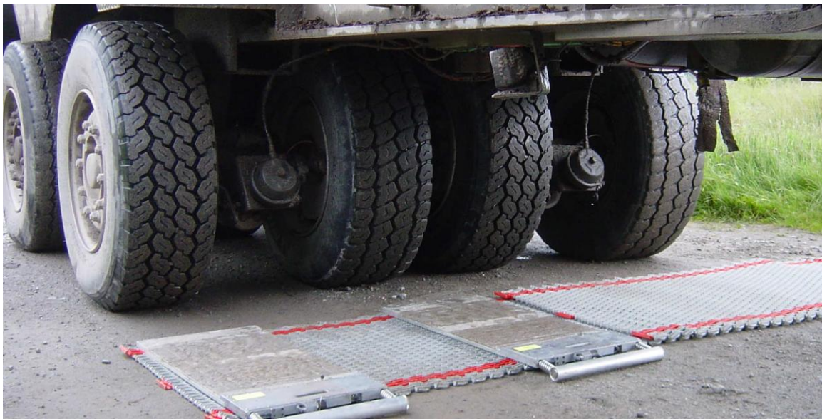
Illustration 10: Weighing King trailer wheels in pairs using mats to compensate for pad thickness
