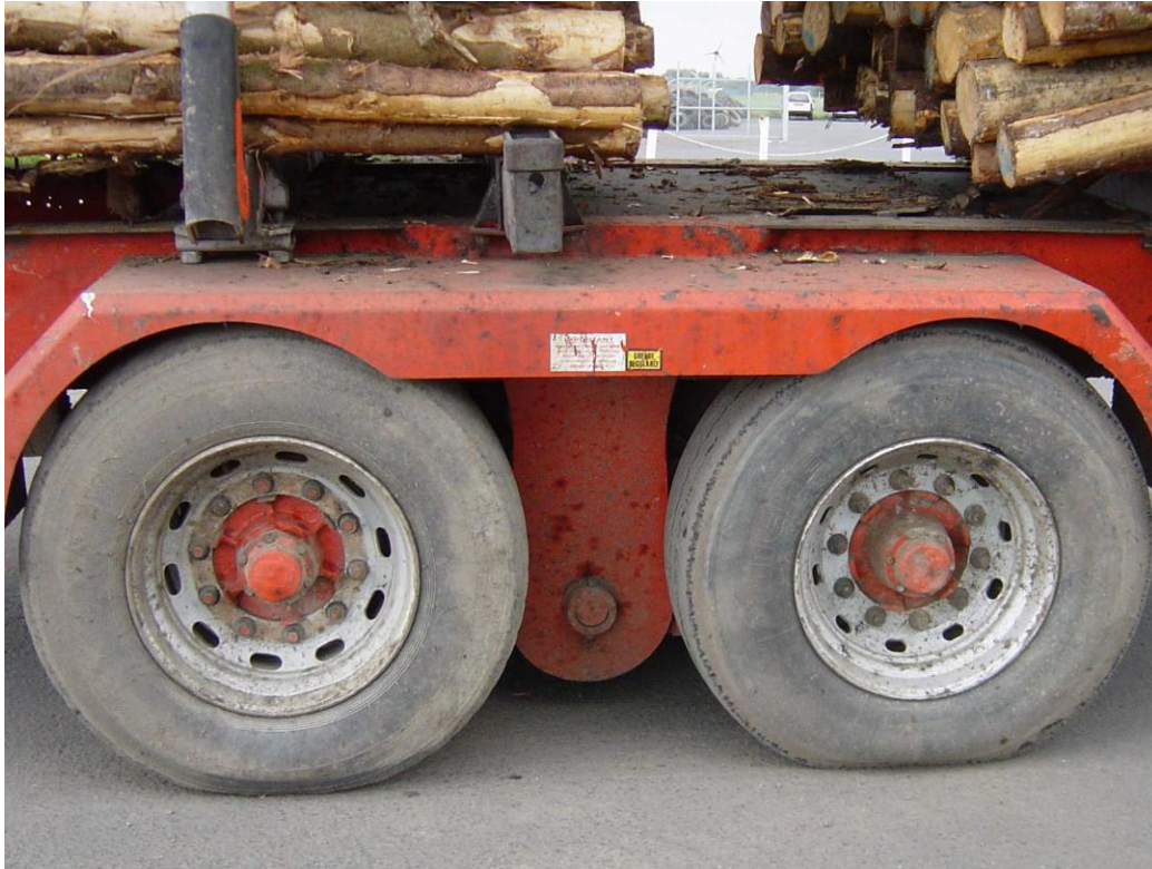
Illustration 8: View of McCauley trailer showing balance beam pivot. Note low tyre pressure
