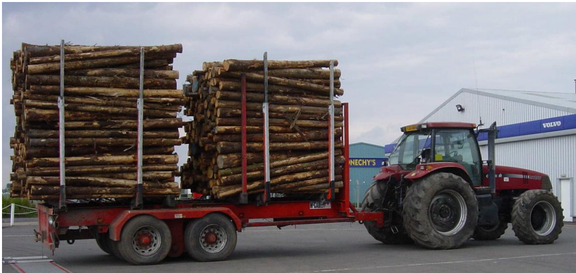
Illustration 11: Fully laden (overloaded) Case trailer being weighed
