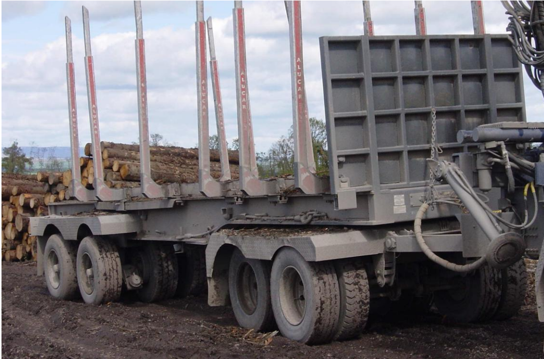
Illustration 6: King trailer showing wheel arrangement. Note inset of bogie rear wheels
